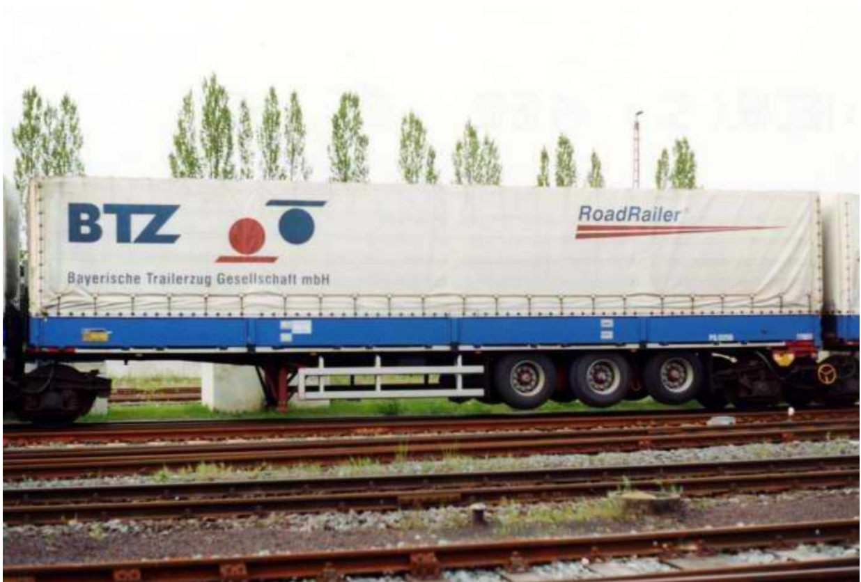
Roadrailer as used by Bayerische Trailerzug (BTZ) until 2003
