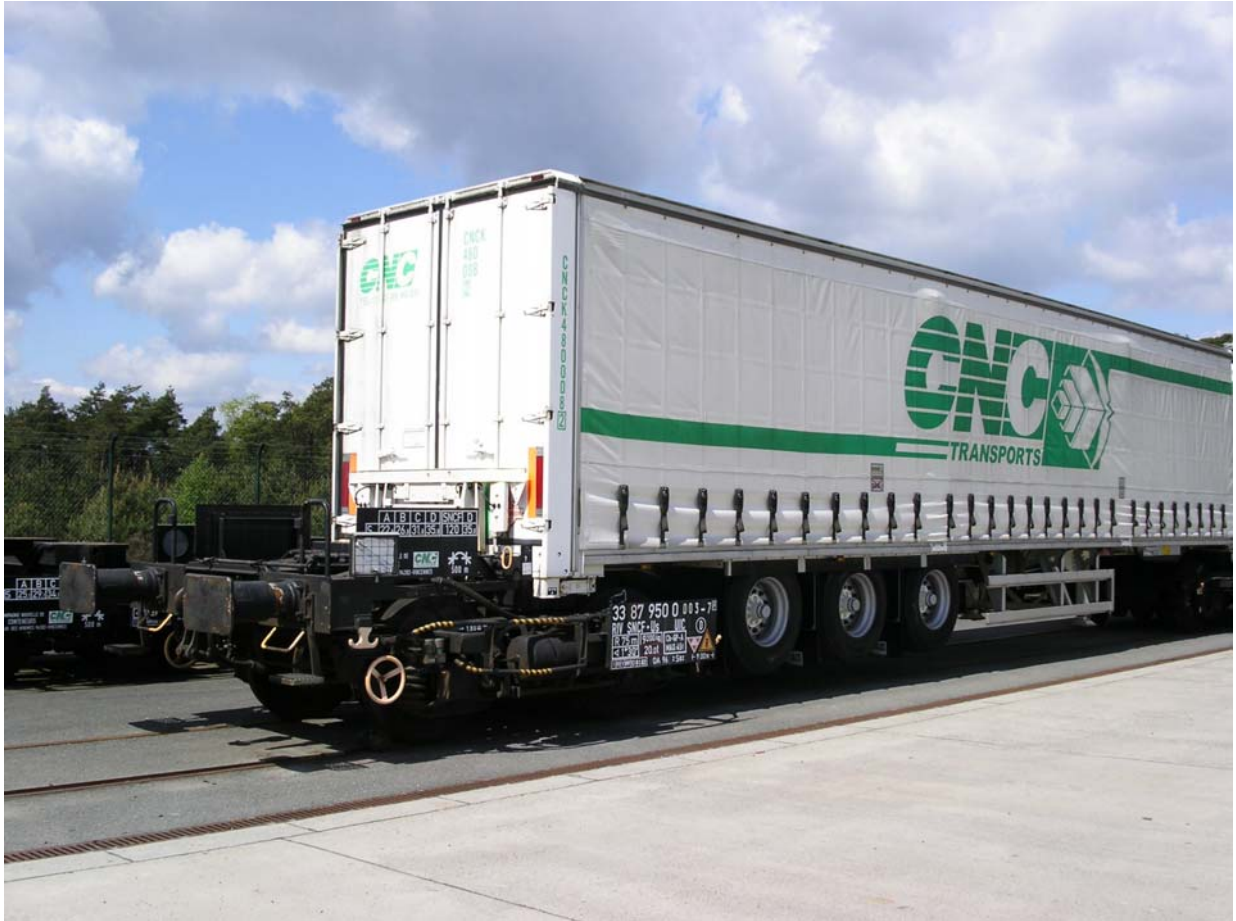
RoadRailer by CNC / SNCF (stored in Soltau, Germany 2005)
