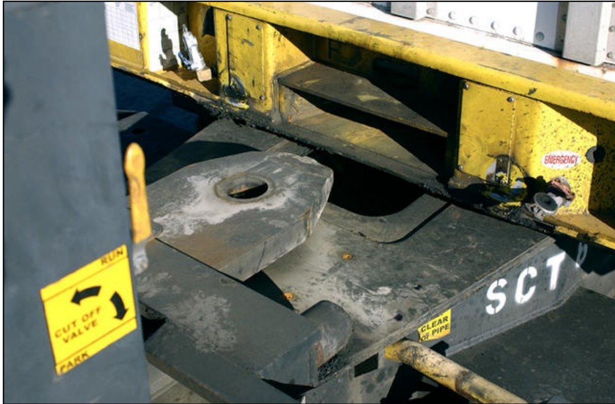
Transition Unit being positioned under Chassis
