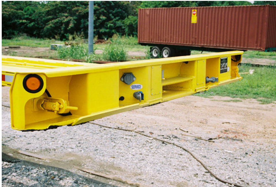
Figura 1 Vista frontal del chasis RailRunner
