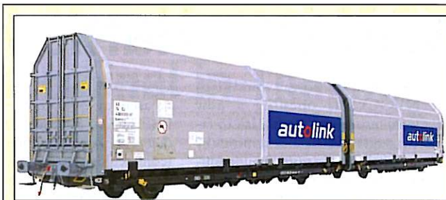
Norway-based Autolink has become the first customer for a new type of railcar developed by Swedish manufacturer Kockums Industrier for the transport of vehicles. The order for 70 twin-coupled wagons, each loading 12 cars is worth SEK 175M. Initial units will be delivered this autumn and all the cars are scheduled to be in operation by the spring of 2009. The new freight cars differ from traditional wagons in several respects. Vehicles are protected by a new type of aluminium roof and sides that can be easily rolled back for loading and unloading. On the return journey, the upper level can be lowered to allow the cars to be loaded with general mixed cargoes on pallets. Autolink transports 75% of all vehicles that are sold in Norway. The new railcars will be used not only in Norway but also throughout Scandinavia for transport from the car plants and import centres to the dealerships as well as between car showrooms
