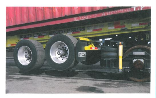
To view and verify the terminal operation at Norfolk & Southern a team of BIC experts was recently invited to see the Calumet terminal in Chicago. They found a most interesting innovation of intermodal transport, operating a commercially successful shuttle service. The technical solution is impressive: Robust for daily use in the railway environment with interesting technical features like
