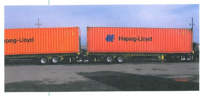
A most interesting innovation in intermodal road-rail transportation is represented by the bi-modal system offered by RailRunner N.A., Inc.: Standard trailer chassis can run over the road, coupled to any standard truck, and also be assembled to a train using special bogies that are provided at the intermodal terminal. This road-to-rail transfer does not need heavy equipment such as gantry cranes or reach stackers and can be performed in some 3 minutes time per unit and then coupled to a train.
