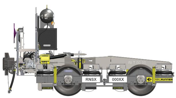
The RailRunner Transition Unit (TU) provides the means of coupling RailRunner containers/chassis to standard locomotives and railcars equipped with conventional railroad knuckle couplers. Equipped with both a RailRunner coupler and a standard knuckle coupler, the TU is first attached to the lead RailRunner chassis/container before coupling with the locomotive or railcar.
