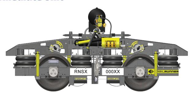
RailRunner's Intermediate Unit (IU) is an integral part of the unique bi-modal system. This bogie transforms the RailRunner chassis and/or road vehicle from highway equipment to a high-speed rail vehicle.
